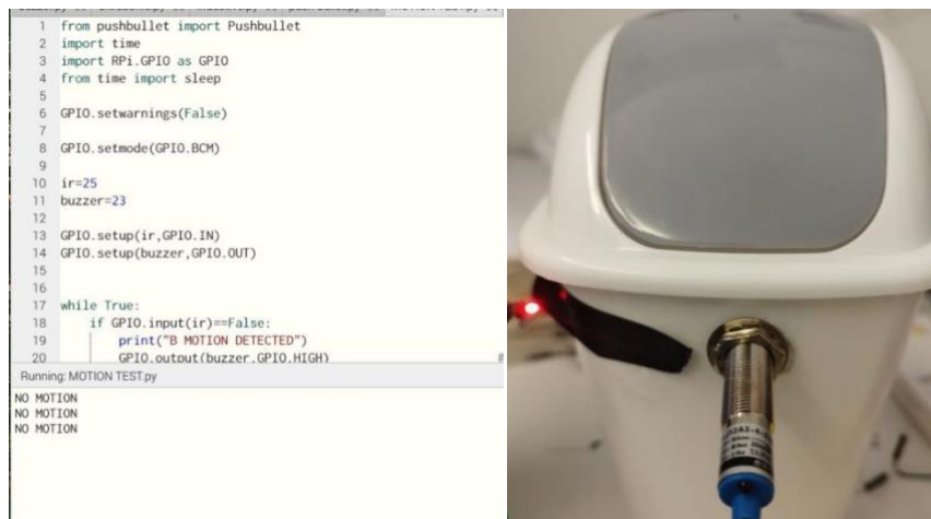
Figure 12. No Motion is Detected When No Metal-Object is Inserted in the Garbage Bin 2
