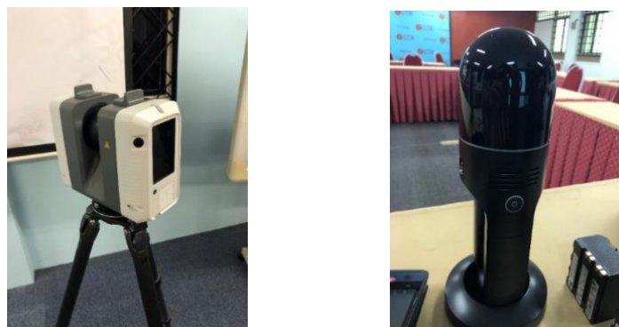
Figure 6. On the left is the Leica RTC360 and on the right is Leica BLK2GO Handheld Laser Scanner
