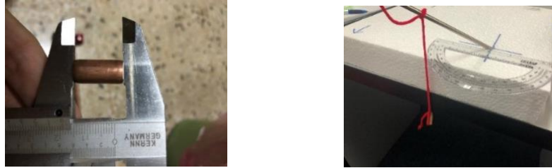
Figure 3. On the left, the measurement of bullet cartridge using Vernier caliper, on the right, measuring the bullet trajectory horizontal component.
