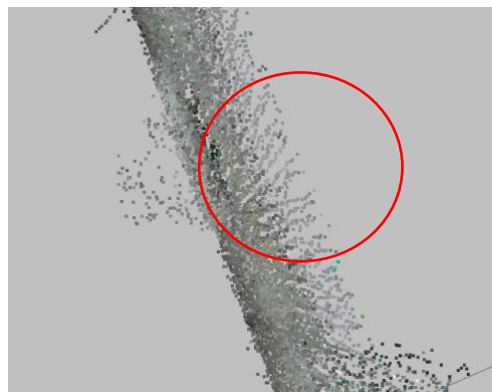
Figure 7. Bullet trajectory at bullet hole 4 and 5. Scanned using BLK2GO Handheld Laser Scanner
